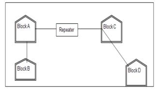
In both the layouts, a hub/switch each would be needed in all the blocks, to interconnect the group of cables from the different computers in each block
