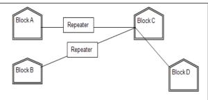
**For layout 2,** since the distance between Blocks A and C is large so a repeater would ideally be placed in between this path
