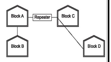
(ii) In both the layouts, a hub/switch each would be needed in all the blocks, to interconnect the group of cables from the different computers in each block.
